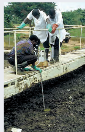
Measuring the scum layer in a faecal sludge pond in Achimota, Ghana. Photo: Eawag/Sandec
